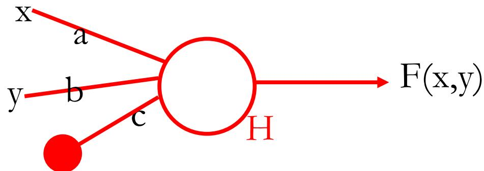
$$\begin{aligned} F(x,y) &= H(ax+by+c) = 1 \\ &= 1 \text{ si } ax+by+c \geq 0, \\ \text{et } 0 \text{ sinon} \end{aligned}$$
